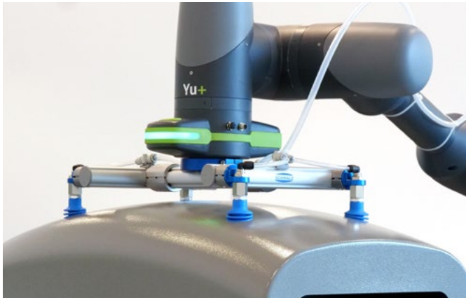
Gripper kit PXT handling a housing cover
